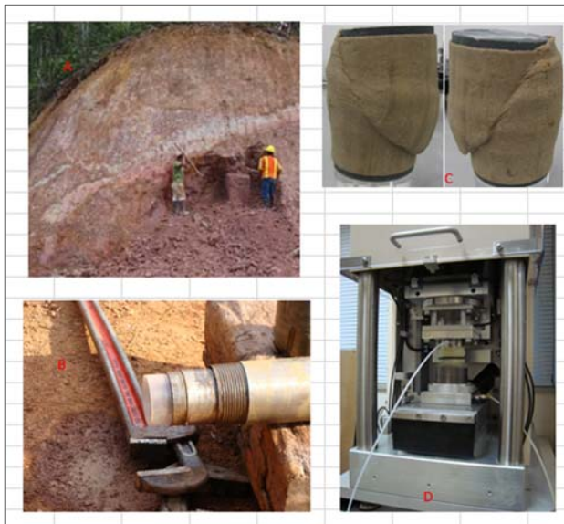
Figure 4. Typical Sampling and Testing Conditions a) Preparation for Block Sample b) Mazier Sample c) Triaxial sample post Tx UU Test and d) A Simple Shear Setup
