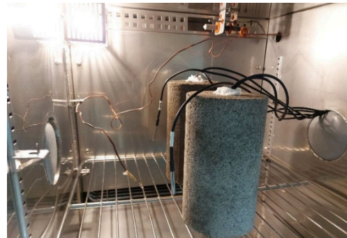
Figure 3. Test setup to simulate outside temperature to find time lag and decrement factor
