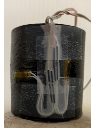
Figure 4. Rubber sample with attached strain gauges
