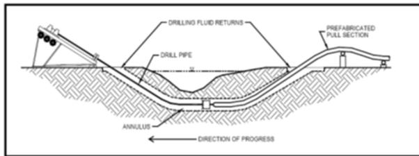
Figure 2. Pullback phase of an HDD (J.D. Hair, 2015)
