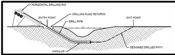
Figure 1. Pilot hole phase of an HDD (J.D. Hair, 2015)
