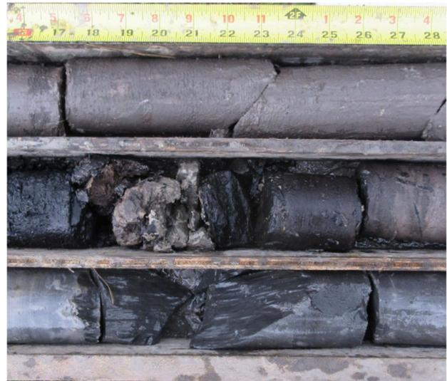
Figure 4. A slickenside feature found in the bottom core run (photo taken by author)
