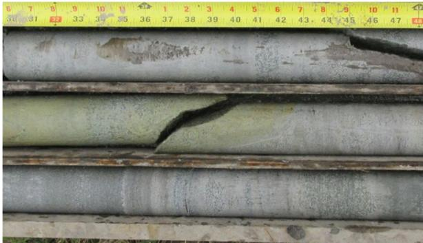
Figure 5: A fracture in discolored sandstone (photo taken by author)
