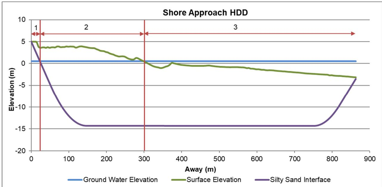
Figure 3. An example of a shore approach HDD profile (example by author)
