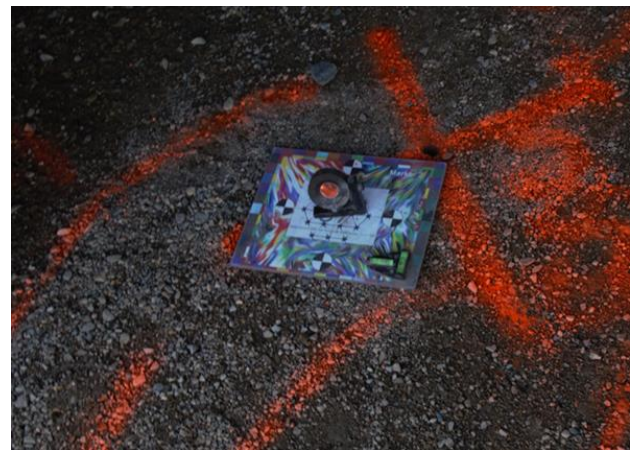
Figure 2: Targets equipped with prisms used to georeference photogrammetry models.
