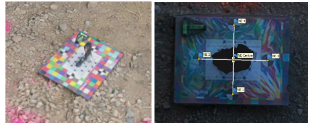
Figure 5: The inaccuracies of the prism (left) and the method to obtain the proper coordinate of the prism (Right).
