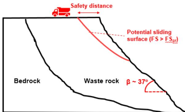
Figure 1. Definition of the safety distance for machinery in end/push-dumping construction for the deposition of waste rock.
