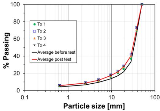
Figure 3. Initial and final particle size distributions of the tested specimens.
