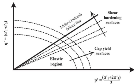
Figure 6. Yield surfaces for the shear strain hardening and volumetric strain (cap) hardening used with the HS model (Surarak et al., 2012).
