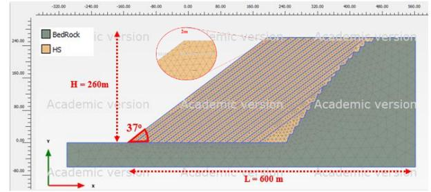
Figure 9. Base case geometry, meshing, and 18 construction stages in the Plaxis model.
