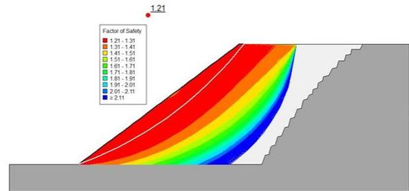
Figure 11. Results from the base case (260 m WRP) analysis in Slope/W; the isocontours show zones with different  $FS$ , with the critical slip surface ( $FS = 1.21$ ).
