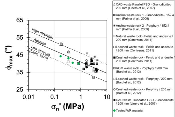
Figure 5. Internal friction angle vs normal stress (modified from Ovalle et al., 2020).
