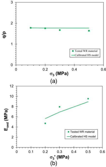
Figure 8. HS Calibration (a) Stress ratio ( $q/p$ ) vs  $\sigma_3$  for tested WR material. (b) Oedometric stiffness vs  $\sigma_3$ .
