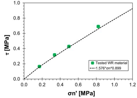
Figure 10. Shear stress  $\tau$  vs  $\sigma_n'$  for tested WR (slightly non-linear relationship with test results).
