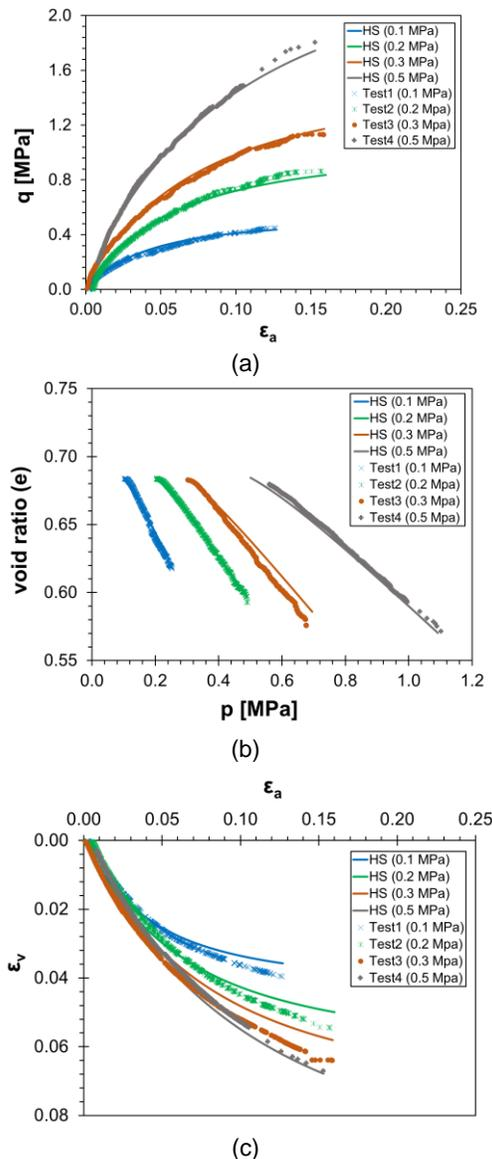
Figure 4. Stress-strain triaxial test results and HS model simulations with calibrated parameters.
