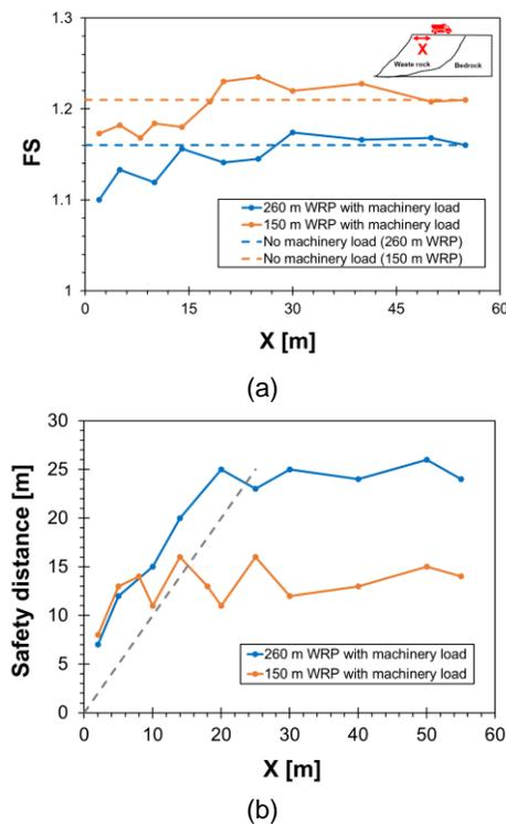
Figure 15. Effect of machinery's load location on variation of (a)  $FS$  and (b) safety distance (the distance between critical slip surface and edge of the WRP).
