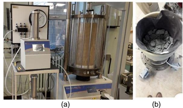
Figure 2. (a) Triaxial compression testing device available at Polytechnique Montreal (b) 300/600 mm WR specimen tested.
