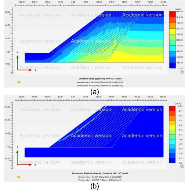
Figure 12. Plaxis simulation results: (a) total deviatoric stress  $q$  distribution after the 18<sup>th</sup> construction stage, (b) most critical slip surface obtained for the base case after a slope stability analysis with the RS method ( $FS = 1.16$ ).
