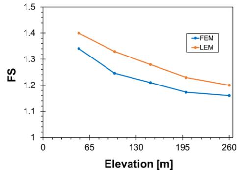
Figure 13. Variation of  $FS$  vs elevation of the modeled WRPs, obtained with the two methods of analysis.
