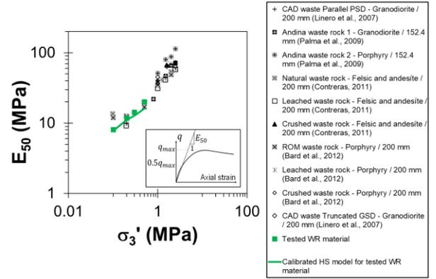
Figure 7. Comparison of  $E_{50}$  vs  $\sigma_3$  for different WR and Rockfill materials (modified from Ovalle et al., 2020).
