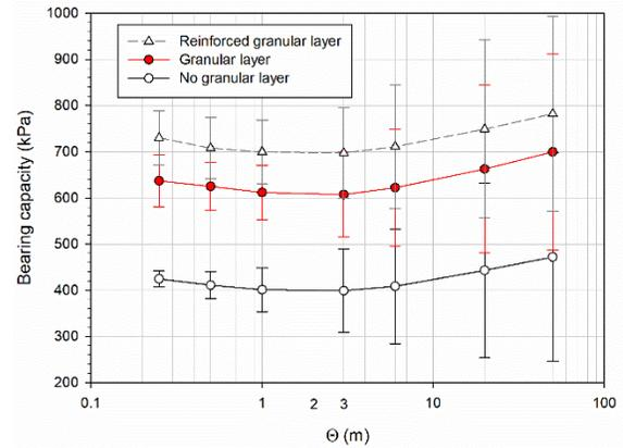
Figure 7. Comparison of mean and spread in computed bearing capacity for different foundation cases and range of isotropic correlation length. Range bars are  $\pm$  two standard deviations.
