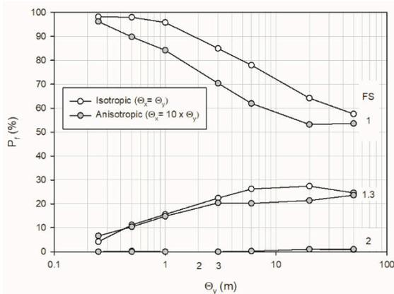
Figure 6. Probability of bearing capacity failure for footing on reinforced granular layer overlying cohesive soil versus isotropic and (vertical) anisotropic spatial variability (correlation length) and different reference deterministic factors of safety.
