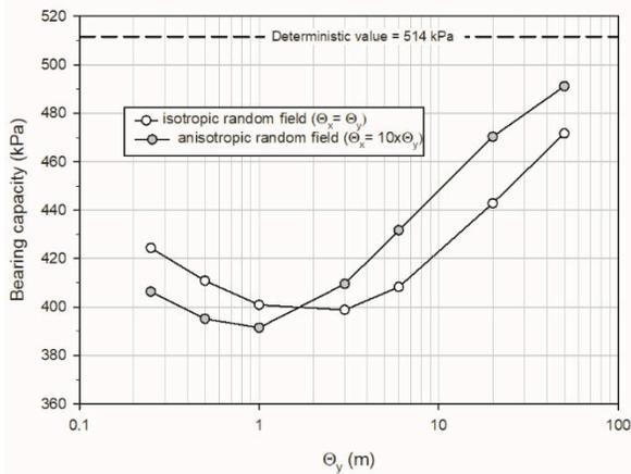
Figure 3. Mean bearing capacity versus correlation length ( $\Theta$ ) for isotropic and anisotropic spatial variability for case of footing seated directly on clay foundation.
