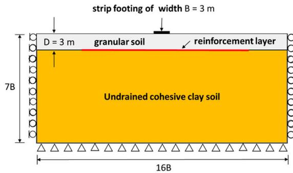
Figure 1. Strip footing seated on reinforced granular base over undrained cohesive clay soil foundation.
