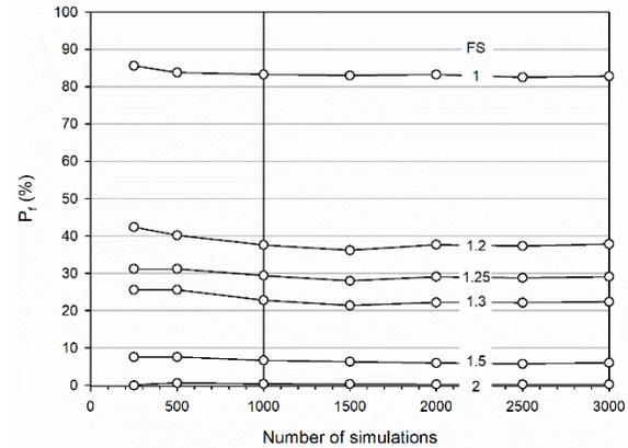
Figure 2. Sensitivity of probability failure ( $P_f$ ) to number of MC simulations for FS = 1 to 2 and footing placed directly on cohesive soil foundation with random variables  $E_u$  and  $s_u$  with COV = 0.5.
