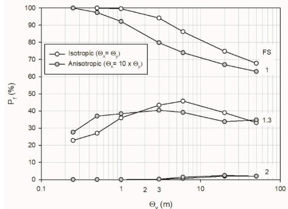
Figure 5. Probability of bearing capacity failure for footing on granular layer overlying cohesive soil versus isotropic and (vertical) anisotropic spatial variability (correlation length) and different reference deterministic factors of safety.
