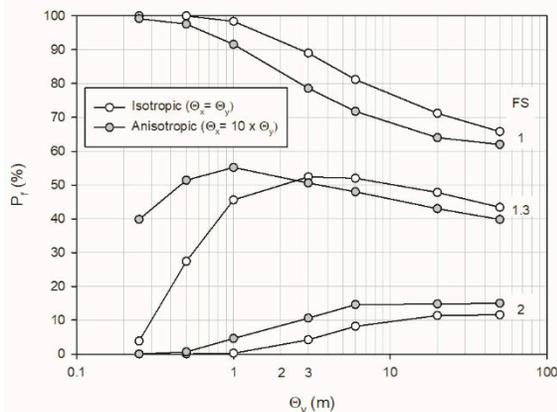
Figure 4. Probability of bearing capacity failure for footing on cohesive soil versus isotropic and (vertical) anisotropic spatial variability (correlation length) and different reference deterministic factors of safety.
