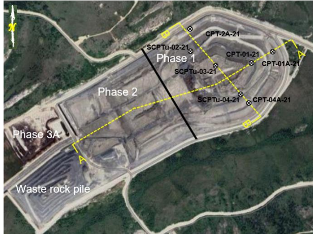
Figure 2. Plan view of the Phase 1 of the Éléonore Mine TSF with selected sections
