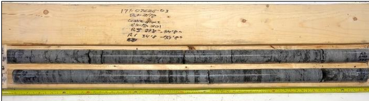
Figure 3: Bedded limestone and shale rock core recovered from one the boreholes.
