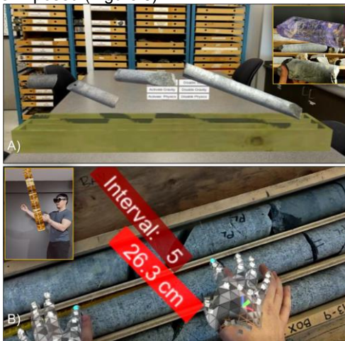
Figure 6. A) Holographic core and B) core sample mapped and measured within MR (Chang, 2021).
