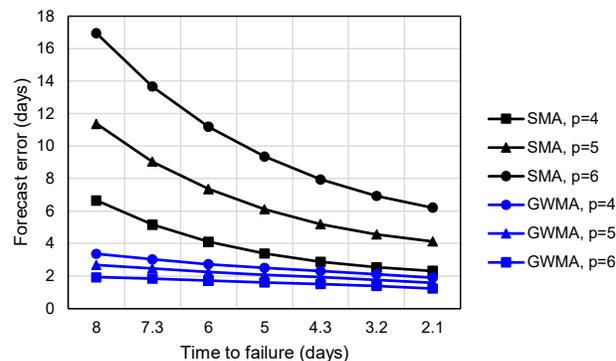
Figure 8. Variation of error in failure time forecast of Mount St. Helens slide using SMA and GWMA at various periods before the failure
