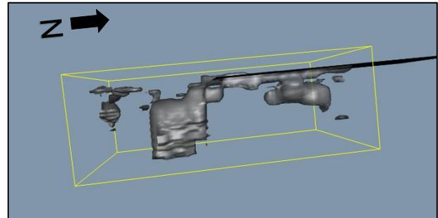
Fig. 6. Side view of the 3D conductivity model shows the delineated conductive anomaly extending to depth below the EM31, below the historical location of the calcium chloride sump. The total depth of the model is 30 meters.
