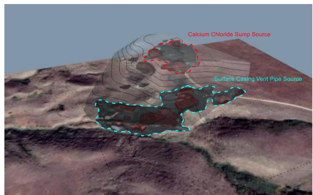
Fig. 10 Interpreted anomalies based on their sources of contamination. Contamination at the top of the hill is interpreted to be sourced from the calcium chloride sump, while down into the coulee is interpreted to be sourced from the leaking surface casing vent pipe.
