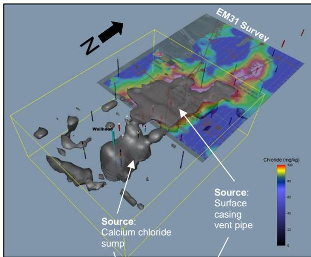
Fig. 5: Looking from the SE corner of the site: A gray isosurface was mapped at 120 mS/m. Note that two main
