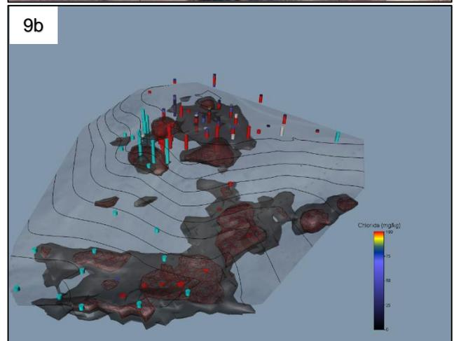
Fig. 9 a) Overview of lease site and lines (yellow) showing rapid ERT lines. b) Pseudo-3D volume showing 120 mS/m isosurface in gray and 150 mS/m isosurface in red. Previously sampled boreholes (pre-2021) are coloured according to chloride concentration (mg/kg). Planned boreholes (2022) informed by RCV results are shown in cyan.
