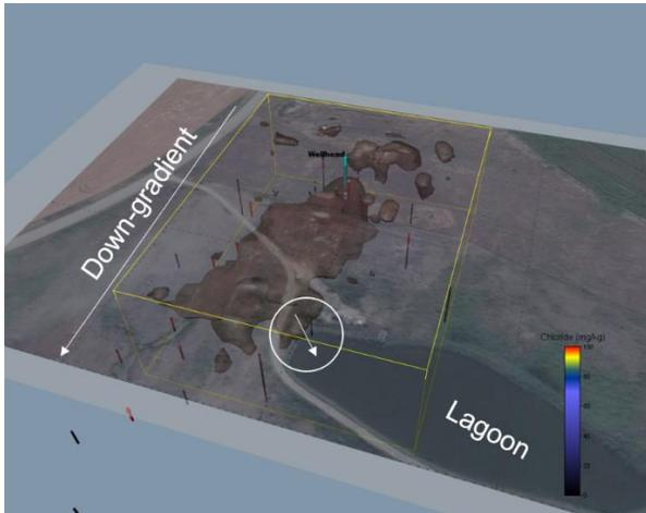
Fig. 8 Perspective view looking from the NW corner of the site. White arrows indicate potential hydraulic pathways for contaminants to flow; down-gradient towards the South Saskatchewan River, and towards the irrigation lagoon.
