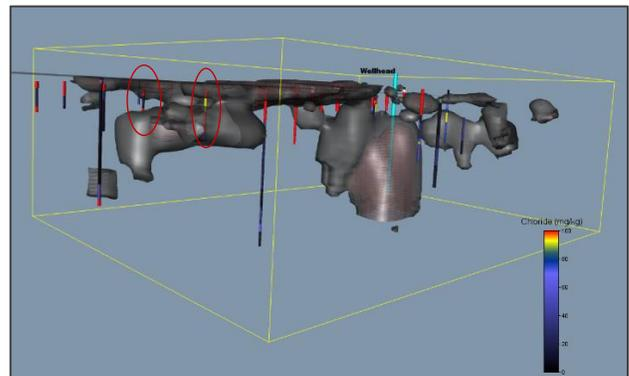
Fig. 7 Perspective view looking from the NW corner of the site: Note the isosurface is widespread at the surface, and steps down to depth below the EM31 surveyed area. Circled in red shows two boreholes that indicate chloride impact at the surface, and at depth with an unimpacted lens of soil in between. The geophysical anomaly matches very well to these geochemical results.
