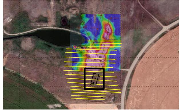
**Fig. 2:** Satellite overview of study site. Yellow lines indicate ERI lines used to build the pseudo-3D volume. A previous EM31 survey is overlain to illustrate the shape of the conductive anomaly (pink = high conductivity, blue = low conductivity). Black lines indicate the historical location of facilities.
