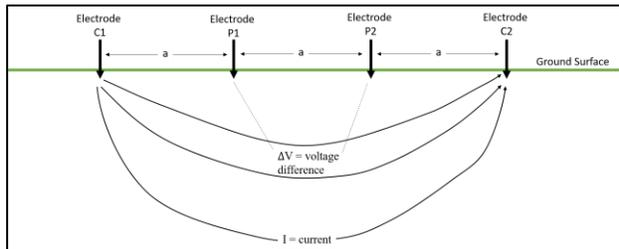
Fig. 4 Typical 4-electrode ‘Wenner’ array deployed on the surface.
