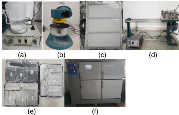
Figure 1. Test block preparation process. (a) Stirring with a magnetic stirrer. (b) Stirring with a mixer. (c) The slurry is poured into the mold. (d) Vibrating with a vibrating table. (e) Test block after 24 hours of demolding. (f) The curing box.
