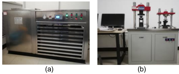
Figure 2. Freeze-thaw cycle testing instrument and strength testing instrument. (a) TDRF-2 concrete rapid freeze-thaw test chamber. (b) Automatic compressive and flexural testing machine.
