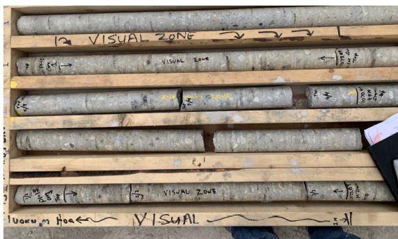
Figure 4. Concrete Core from pile P1-15
