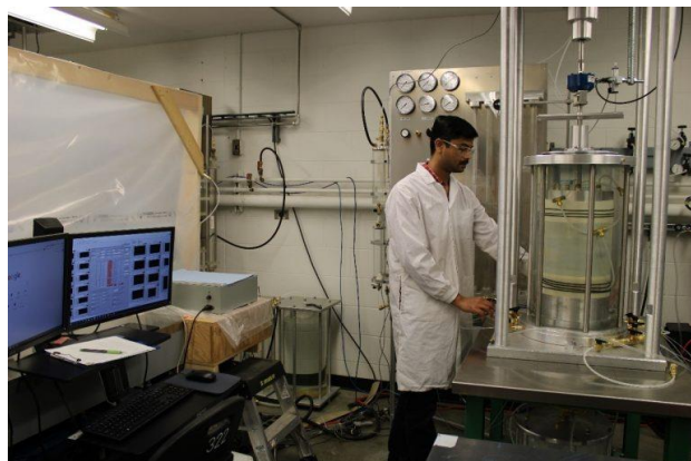
Figure 8. The 200 mm Flexible-wall Permeameter (FXP) of the current study in the UBC graduate soils laboratory
